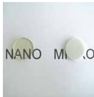
A polymer filled with nanoparticles is clear and translucent, whereas one filled with microfillers, is opaque.
