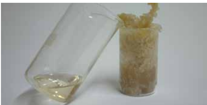
On the right: a resin with 38% micro-filler yields a fissured mass. On the left: the same resin with 40% nano-filler still remains liquid.
