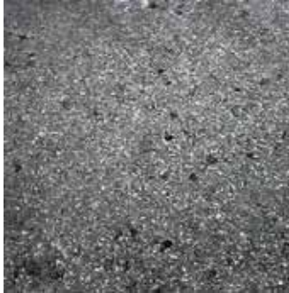
Macro-filler composites are similar to asphalt in that large filler particles can break away from the resin matrix. This is why they are quite difficult to polish.
